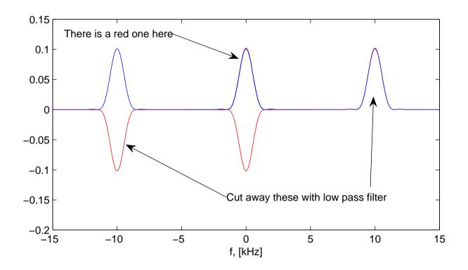
The red spectras around f=0 cancel out, thus, we can detect the blue independently from the red. Equivalent for demodulation with  $\sin(2\pi t f_c)$
