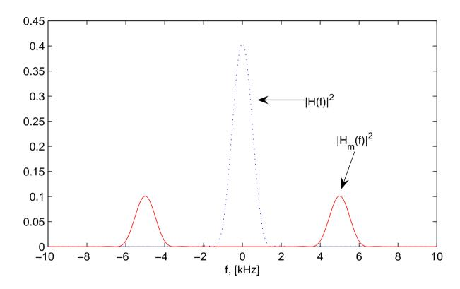
The carrier modulated signal is  $y_m(t) = y(t) \cos(2\pi t f_c)$
