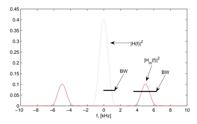
The carrier modulated signal is  $y_m(t) = y(t) \cos(2\pi t f_c)$ But bandwidth gets twice as large!
