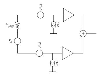
Remember that the  $v_n$ -sources and  $R_{gdiff}$  generates noise at both the amplifier inputs, which furthermore is fully correlated!
