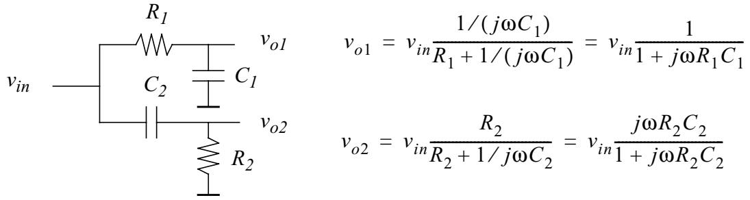
$$\frac{v_{o1}}{v_{o2}} = \frac{1}{j\omega R_2 C_2} \cdot \frac{1 + j\omega R_2 C_2}{1 + j\omega R_1 C_1} = \{R_1 C_1 = R_2 C_2 = RC\} = \frac{1}{j\omega RC}$$
