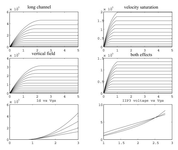
The two plots in the bottom are extras. They show how Id and IIP3 vs Vgs looks for the four cases. One case is omitted in the IIP3 plot, since in the long channel case IIP3 is infinite.
