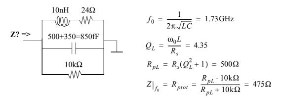
With more metal layers, a higher Q and/or lower parasitic capacitance can be achieved.
