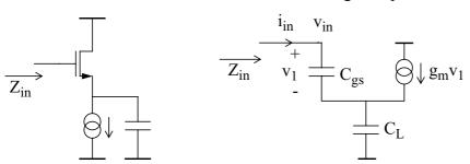
$$\begin{cases} g_m(v_{in}-v_{out})+(v_{in}-v_{out})sC_{gs}-v_{out}sC_L=0 \Rightarrow v_{in}(g_m+sC_{gs})=v_{out}(g_m+sC_{gs}+sC_L)\\ i_{in}=(v_{in}-v_{out})sC_{gs} \end{cases}$$
