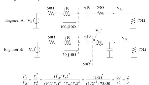
I solution A the load seen by the source is 100-j $10\Omega$ , instead of the optimal 50-j $10\Omega$  of solution B. Furthermore, signal power is wasted in the extra  $25\Omega$  resistor. One third of the power is lost in A, compared to the optimal solution in B. (The series connected capacitor and inductor of B can be combined in just one component).
