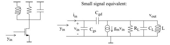
The negative real part of  $y_{in}$  occurs due to  $C_{gd}$  and the load being inductive at some frequencies. To simplify the calculations, assume  $C_{gd} << C_L$ , so that the influence of  $C_{gd}$  on the voltage gain can be disregarded:
