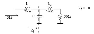
$$\begin{split} R_I &= 300\Omega \Rightarrow Q = Q_{left} + Q_{right} = 7.68 + 2.24 = 9.92 \Rightarrow \text{close enough} \\ C &= \frac{Q}{\omega R_I} = 52 \text{pF} \qquad L_1 = \frac{Q_{left} \cdot R_{prim}}{\omega} = 6.1 \text{nH} \qquad L_2 = \frac{Q_{right} \cdot R_L}{\omega} = 18 \text{nH} \\ \hat{I_{L_1}} &= \frac{\hat{V}_{prim}}{R_{prim}} = 0.63 \text{A} \qquad \hat{I_{L_2}} = \frac{\hat{V}_L}{R_L} = 0.20 \text{A} \end{split}$$
