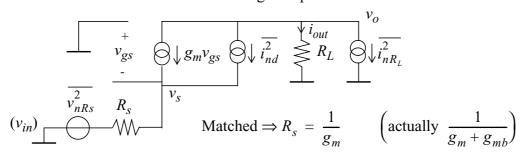
All noise sources are transformed to the output and then compared in order to find F.
