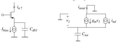
$$\begin{split} g_{m} \cdot v_{1} + i_{nd} + v_{1} \cdot sC_{tot} &= 0 \Rightarrow v_{1} = -\frac{i_{nd}}{g_{m} + sC_{tot}} \\ i_{nout} &= i_{nd} + g_{m} \cdot v_{1} = i_{nd} \cdot \left(1 - \frac{g_{m}}{g_{m} + sC_{tot}}\right) = i_{nd} \cdot \frac{sC_{tot}}{g_{m} + sC_{tot}} \\ \overline{i_{nout}^{2}} &= \overline{i_{nd}^{2}} \cdot \left(\frac{sC_{tot}}{g_{m} + sC_{tot}}\right)^{2} = \overline{i_{nd}^{2}} \cdot \left(\frac{j\omega}{g_{m}/C_{tot} + j\omega}\right)^{2} \end{split}$$
