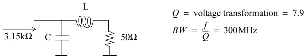
$$L = \frac{QR_L}{\omega_0} = 26\text{nH} \quad C = \frac{1}{\omega_0^2 L} = 170\text{fF}$$
