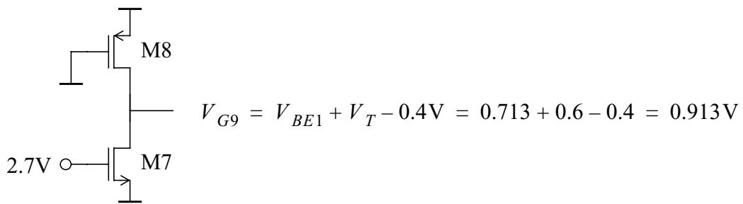
M7 and M8 operate in the triode region with the same drain current:
