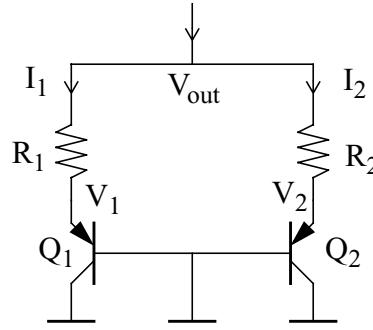
$$I_1 = (V_{out} - V_1) \cdot \frac{1}{R_1} = \left( V_{out} - V_{GO} + V_T \cdot \ln\left(\frac{A_E B T^r}{I_{c1}}\right) \right) \cdot \frac{1}{R_1}$$
