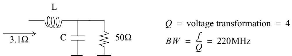
$$L = \frac{QR_{PA}}{\omega_0} = 2.2\text{nH} \quad C = \frac{Q}{\omega_0 R_L}$$
