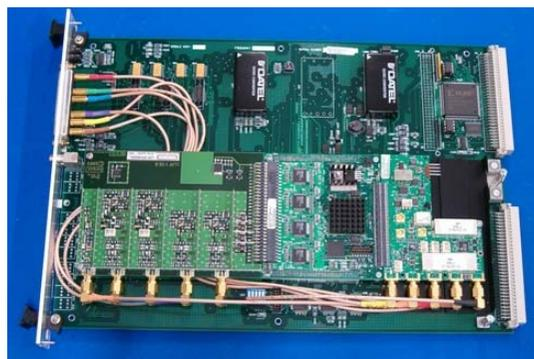
Example: SNS Front end LLRF board (ADC – FPGA – DAC, L. Doolittle et al)
