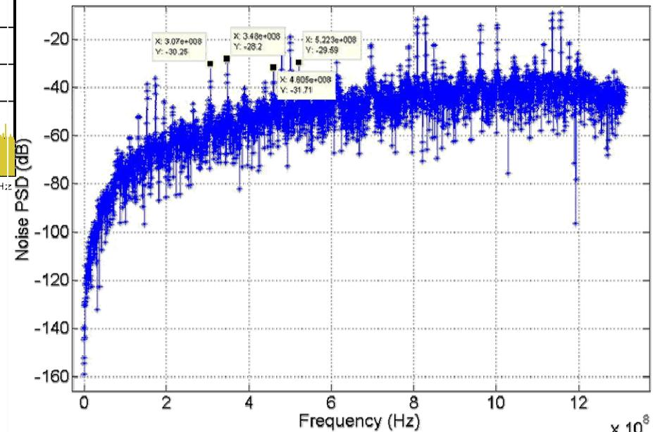
*Simulated  $\Delta\Sigma$  modulator Noise PSD*
