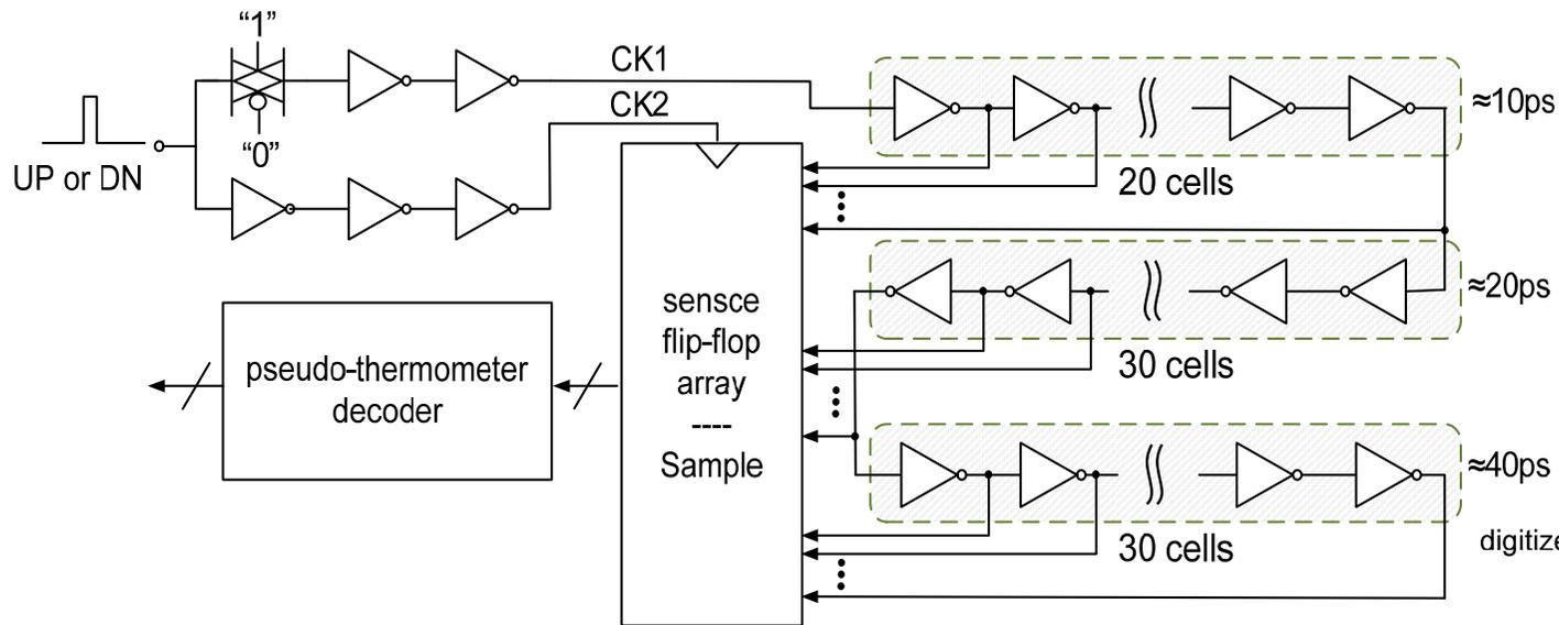
**TDC with uneven delay cells**
