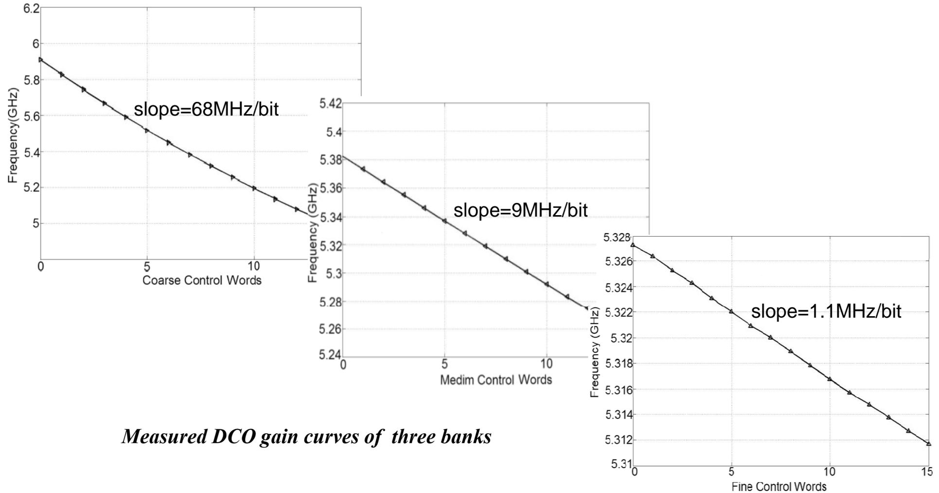
*Measured DCO gain curves of three banks*
