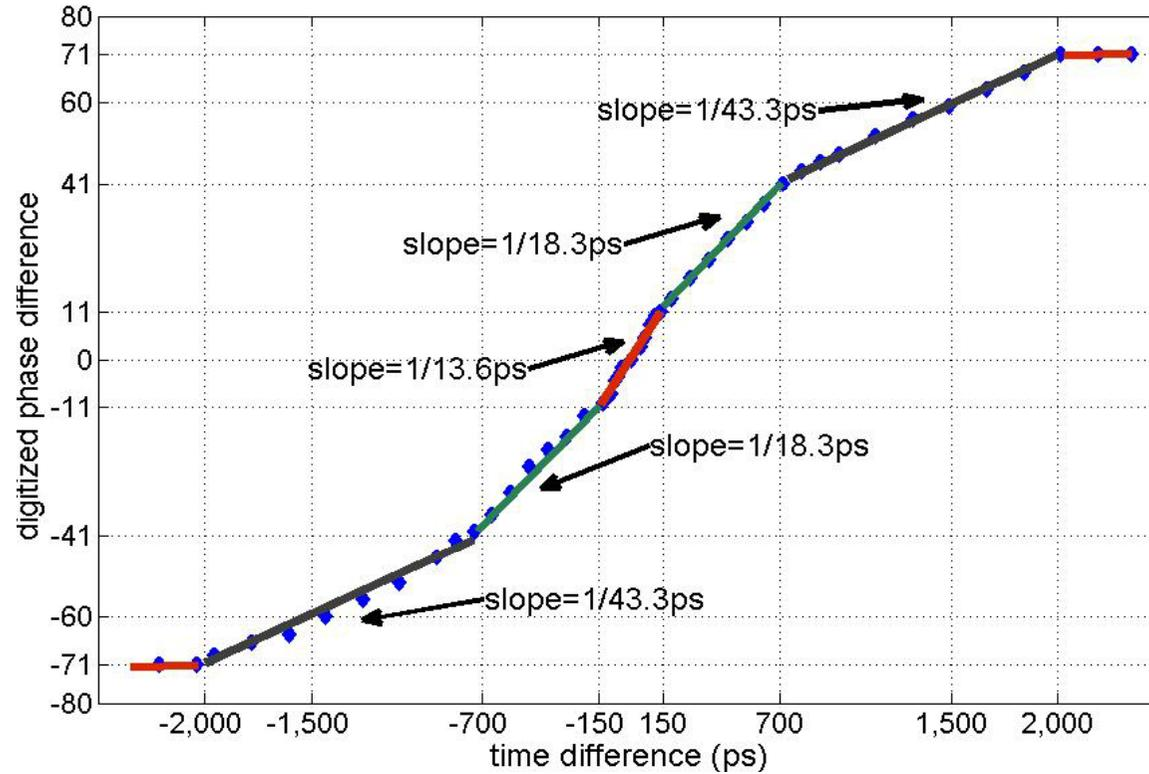
*Measured characteristic of Uneven-cell TDC*
