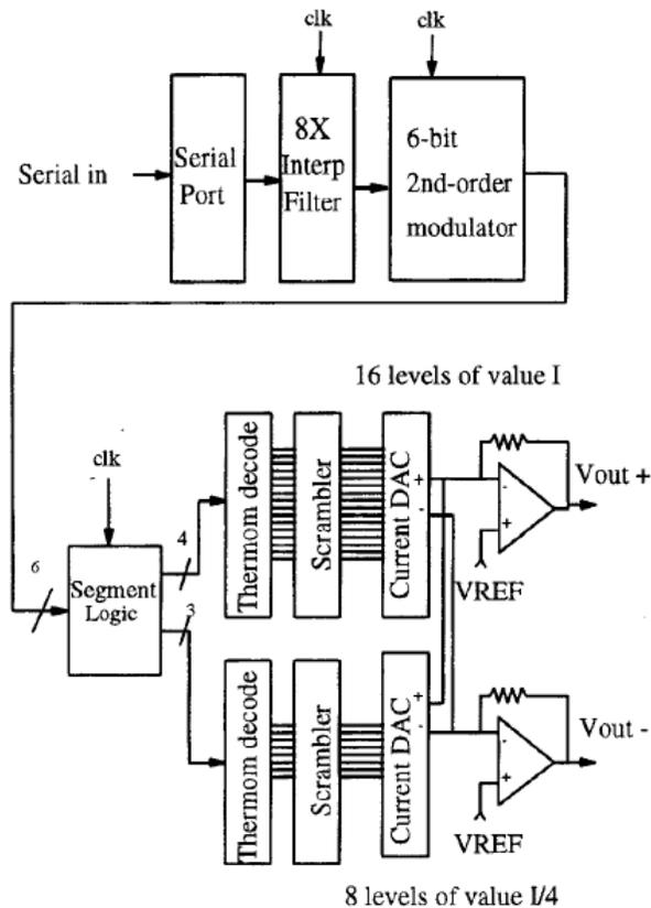
Figure 1: Chip block diagram (1 channel of 2).
