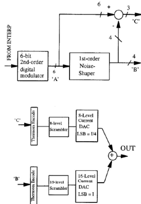
Figure 2: Noise-shaped segmentation circuit.
