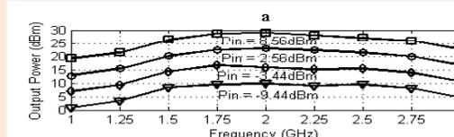
PA Frequency Response, Output Power (a), Power-Added Efficiency (b)
