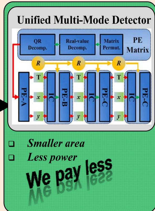
Detect **multi-mode MIMO** signal with **smaller area** and **less power**
