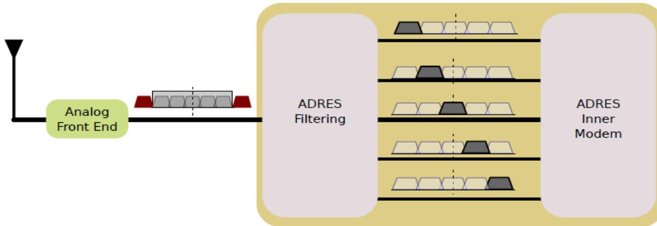
FULL SDR FILTERING: ADRES Filtering + ADRES Inner modem
