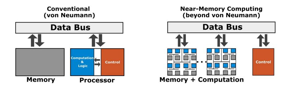
NMC architecture realized as co-processor integrated in a microcontroller unit (MCU) cache memory using SRAM
