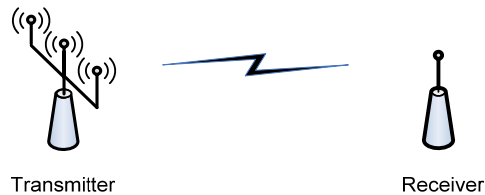
Figure 2.4 A multiple input - single output system.
