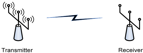
Figure 2.7 A multiple input - multiple output system.
