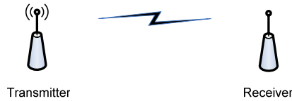
Figure 2.1 A conventional SISO communications system.
