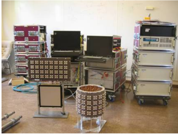
Figure 5.2 Channel sounder system and antennas.
