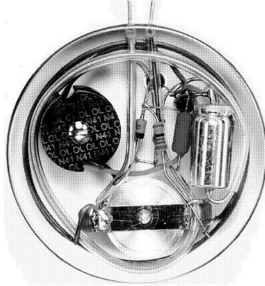
Figure 6: A replica of the first implanted pacemaker molded in a shoe-polish can.
