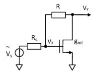
Fig. 18. CS LNA with resistive feedback
