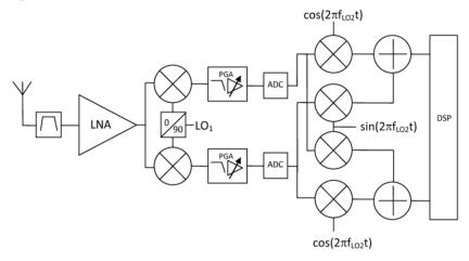
Fig. 10. Architecture of the low-IF receiver
