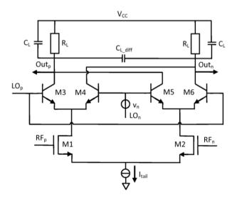
Fig. 25. Double balanced BiCMOS active mixer
