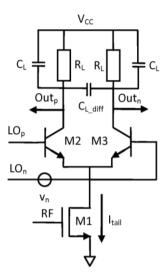
Fig. 24. Single-balanced active BiCMOS mixer
