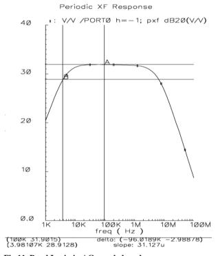
Fig.11. Band I gain in AC-coupled mode
