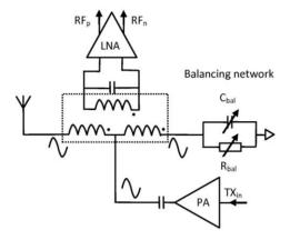
Fig. 33. Architecture using electrical balance to cancel the TX signal
