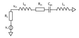
Fig. 12. Model for input matching Q-value calculation
