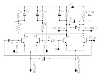
Fig.5. Switching mixer core
