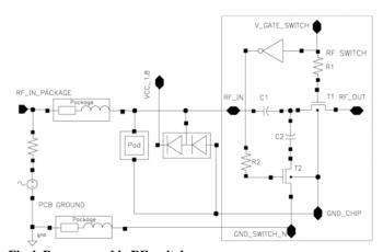
Fig.4. Programmable RF switch
