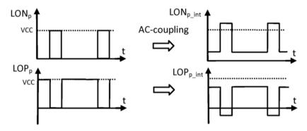
Fig. 31. AC coupling of the four-phase clock to increase the switch overdrive voltage
