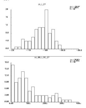
Fig.13. Band I histogram of I-mixer  $IM_2$  in  $dBV_p$  and DC-offset at the differential mixer output versus iteration number with the mixer feedback loop on
