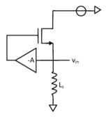
Fig. 16. Common-gate LNA with g<sub>m</sub>-boosting feedback
