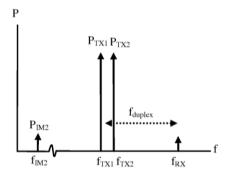
Fig. 3. Second order distortion with AM modulated TX-leakage
