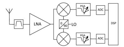
Fig. 9. Architecture of the zero-IF receiver
