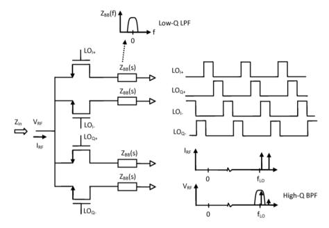
Fig. 32. Current-driven passive mixer with four-phase clock and frequency translation of  $Z_{BB}$
