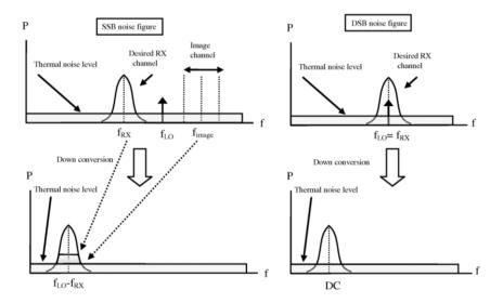
Fig. 2. Single and double sideband noise figure definitions
