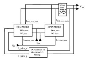
Fig.3. Block diagram of the single ended mixer with IM<sub>2</sub>-suppression
