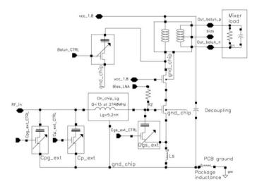
Fig.3. Multiband programmable LNA including tunable balun
