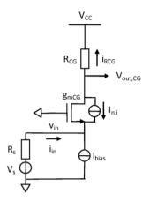
Fig. 23. CS-stage with noise source  $I_{n,i}$
