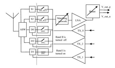
Fig.2. Architecture of the presented multiband single ended LNA
