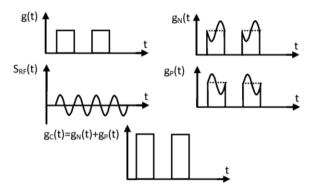
Fig. 27. Switch conductance of the complementary passive mixer
