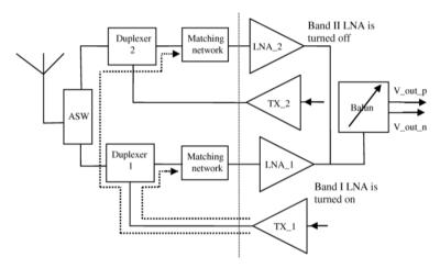
Fig.1. TX-leakage paths in a common multiband LNA
