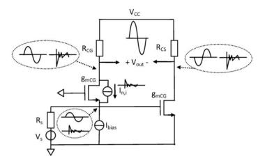
Fig. 22. Noise cancelation with combination of CS- and CG stage
