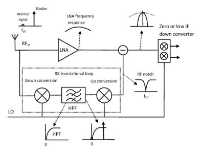
Fig. 34. Feed forward blocker cancelation architecture
