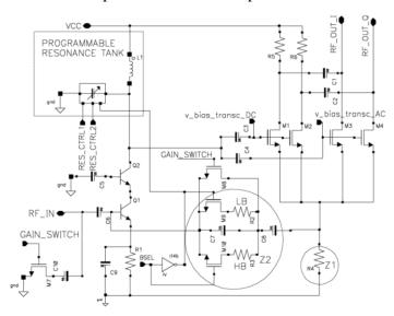
Fig.4. Multiband programmable current-to-current feedback RF amplifier
