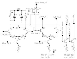
Fig.6. Mixer feedback loop
